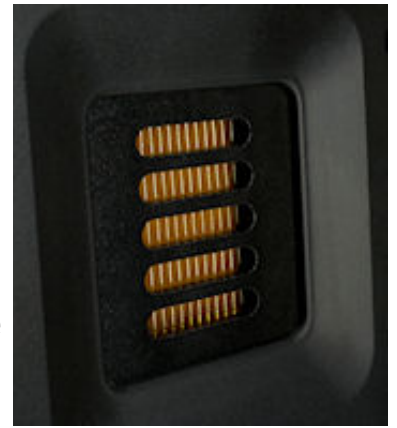
Where the magic happens: the Motion Series' folded motion tweeter.
